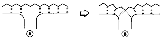
FIG. 1. Conformations of a linear paraffin on the "hilly" surface of a zeolite crystallite. Adsorption (and conversion) is favored for molecules which match best the surface geometry and reach a van der Waals energy minimum. Situations A and B correspond to the molecule without and with the optimization of its interactions with the surface (schematized by the symbols // and ///), respectively.
